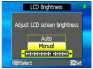
3. For manual adjustment, use the **Left**/ **Right** buttons to adjust the brightness.
